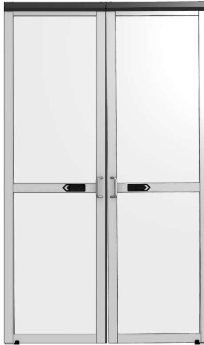
Figure 11. The reveal between the doors is larger at the bottom. Complete steps 2-3 and 6-12, skipping steps 4-5, to adjust the reveal.
