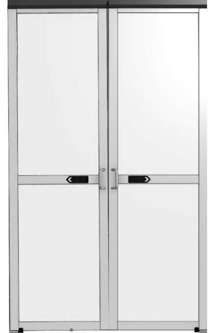
Figure 12. The reveal between the doors is larger at the top. Complete steps 2-12 to adjust the reveal.
