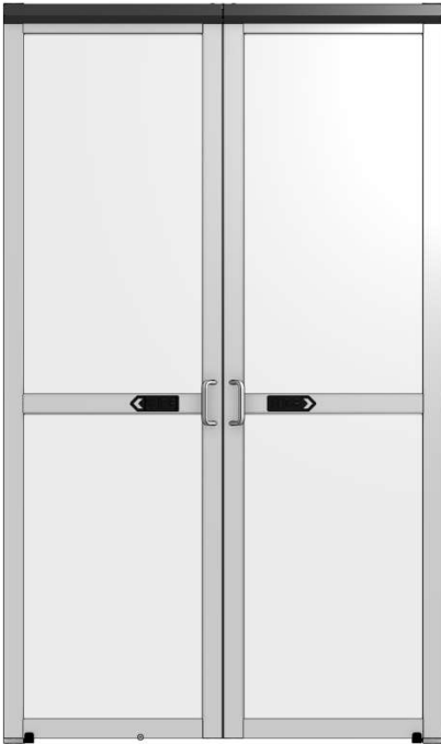
Figure 10. The reveal between the doors is consistent from top to bottom.
