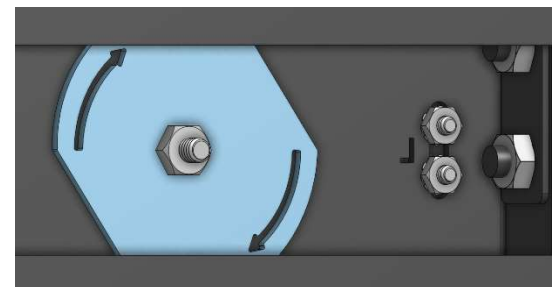
Figure 17. The door slide adjustment cam inside the header adjusts the panel alignment.
