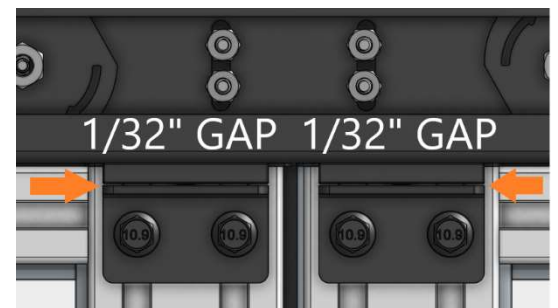
Figure 18. Set the gap between the magnets and latch brackets to approx. 1/32" (8 sheets of paper.)
