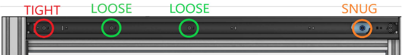
Figure 16. Loosen the intermediate door slide screws, keeping the outermost screw tight and the adjustment cam screw snug.
