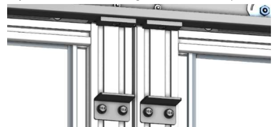
Figure 14. Slide magnetic brackets downward.
