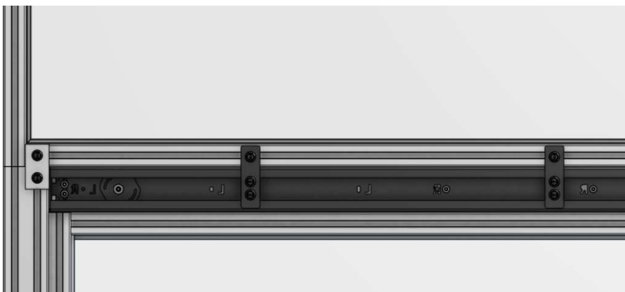
Figure 8. Always fasten over-door panels at no less than 2 mounting positions.
