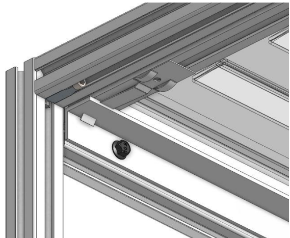
Figure 10. Fixing Roof Panel with Ludwig Clips
